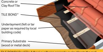
TILE BOND<sup>™</sup> Roof Tile Adhesive adheres concrete or clay tiles to the roof deck/substrate. Refer to tile manufacturer's instructions for details.
