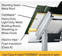
frame designs, where the insulation boards may be left exposed to the interior. Tape top side of seams with WEATHERMATE<sup>™</sup> Straight Flashing.
