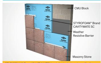
STYROFOAM<sup>™</sup> Brand CAVITYMATE<sup>™</sup> Insulation is designed specifically for moist cavity wall environments. Manufactured with distinct carbon block technology to absorb infrared radiation, STYROFOAM<sup>™</sup> Brand CAVITYMATE<sup>™</sup> Ultra Insulation has an R-value of 5.6 per inch - the highest of any polystyrene foam insulation and is available in 15 3/4" and 16" widths making it easy to fit between brick ties in cavity wall applications.
