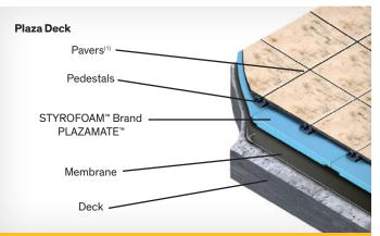
STYROFOAM<sup>™</sup> Brand PLAZAMATE<sup>™</sup> Insulation is designed to hold up under the heavy demands of plaza roof construction. (1) Pavers require pedestals unless STYROFOAM<sup>~</sup> Brand Ribbed ROOFMATE<sup>~</sup> Insulation is used.
