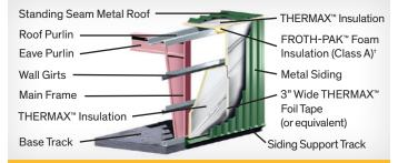
THERMAX<sup>™</sup> Insulation products help safeguard pre-engineered metal buildings against thermal loss and moisture buildup. A variety of thicknesses and lengths up to 30' are available to meet specific design requirements. <sup>™</sup>For air sealing the roof/wall juncture
