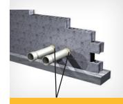
Seal smaller areas, such as gaps around pipe penetrations, with GREAT STUFF PRO<sup>™</sup> Gaps & Cracks Insulating Foam Sealant.
