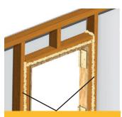
GREAT STUFF PRO<sup>™</sup> Window & Door Insulating Foam Sealant fills gaps around window and door frames without causing bowing, when properly applied.
